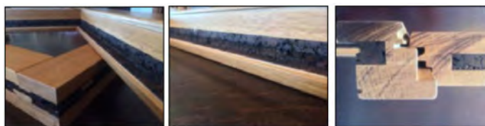
One 20mm Cork layers in a window frame of 500 x 500mm
